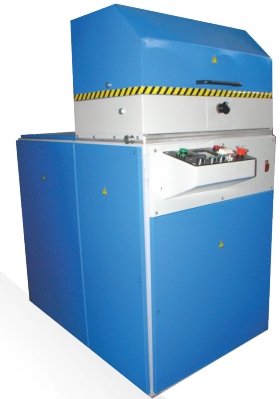
The magnetic-pulse press MIP-10 (MIP-20, MIP-30) with energy output of 10kJ (20 kJ, 30 kJ) and max. total capacity of 10 kW (15 kJ, 20 kJ)
